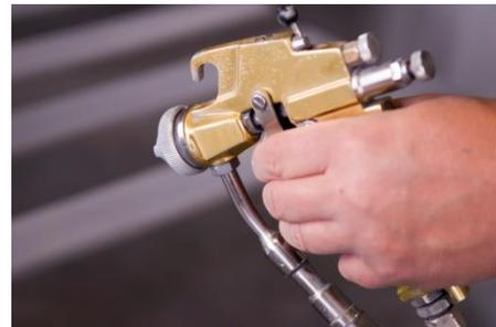
b. Some characteristics of the paint, such as its viscosity, shear when mixing, or tendency to settle can affect how well the paint atomizes, its tendency to dry spray, and rheological properties that could affect your ability to get a uniform, well controlled coating.
