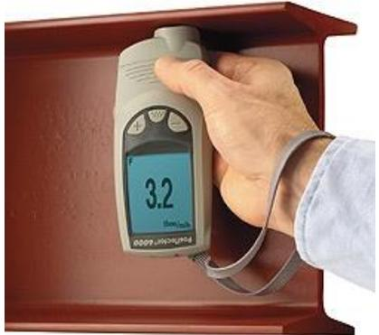
panels of varying different (dry) film thicknesses which are then tested and compared. The goal is to optimize the film thickness for the job at hand. Obviously you don't want to put more paint on the parts than needed, since extra paint costs money without adding much value.
